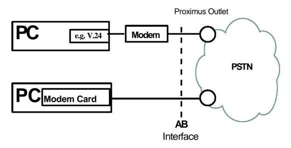
PSTN is used at customer premises to get access to the IP network. In this case, the service supports the following types of transfer :
