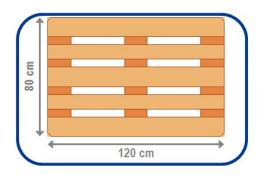
To ensure the stability of the Europallet, the boxes stacked on it must not surpass the 80 x 120 cm base. To prevent a stack from bending or sagging, it can be bound with transparent (shrink) wrap, carton or wooden planks to protect the corners, which can also be bound by elastic straps or rope.
